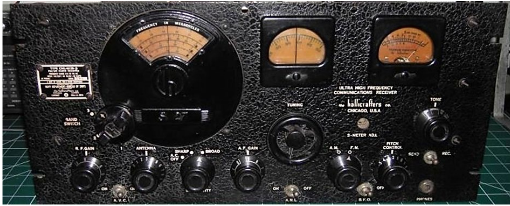
The S-27 receiver covered 27.8 to 143 MHz (Photo courtesy UK Vintage Radio web page)
