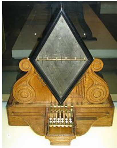
Cooke and Wheatstone's five-needle telegraph from 1837
