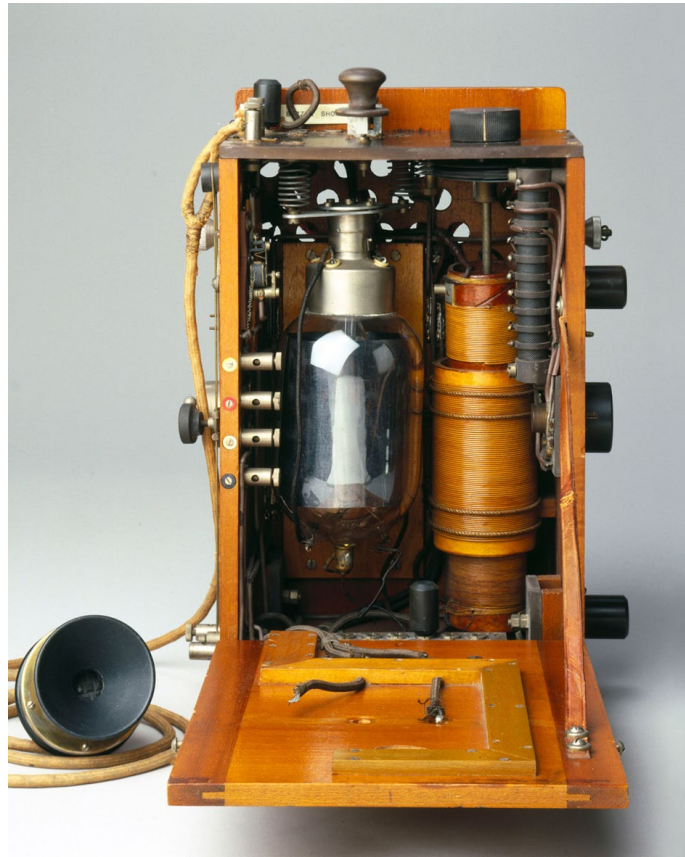
Marconi engineers serving in the British Royal Flying Corps developed this aerial telephony set.
