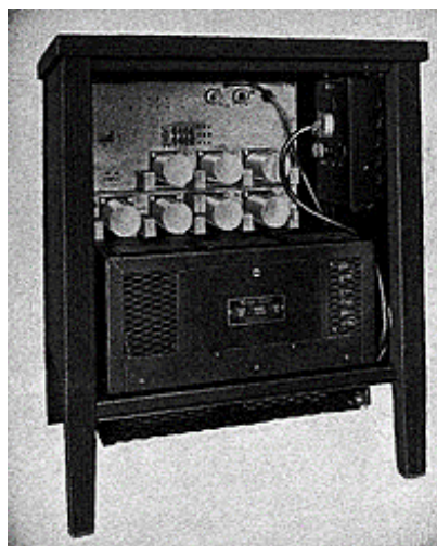
Bell 131B2 mixer, used to XOR teleprinter signals with one-time tapes, was the first device from which classified plain text was extracted using radiated signals.
