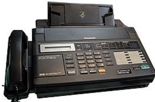
Fax machine from 1990, using thermal printing which required special, relatively expensive thermal paper.
